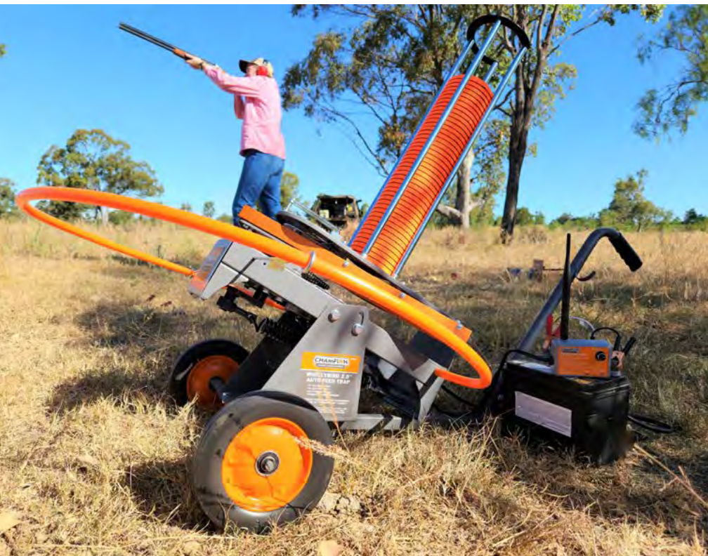
WheelyBird 2.0 connected to portable 12volt battery and wireless remote release ready to go.
