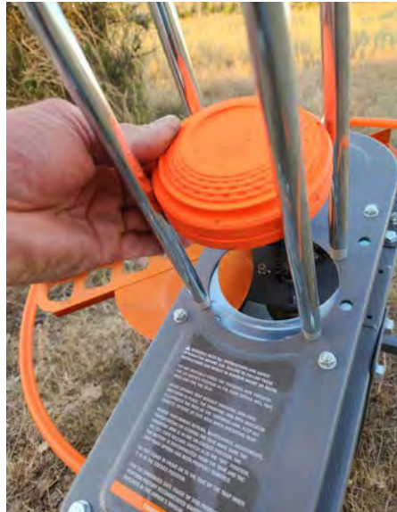
The WheelyBird 2.0 must be in the uncocked position prior to loading clays.
