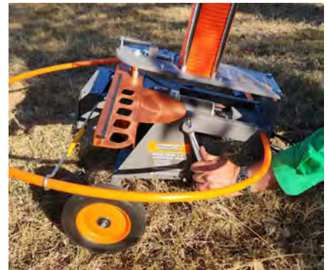
Changing the clay trajectory done safely by disconnecting the battery and easily with a spanner.
