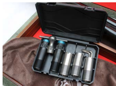
There are seven choke tubes supplied, including two longer 72mm being half- and full-chokes along with a sturdy propeller-type choke tube spanner.
