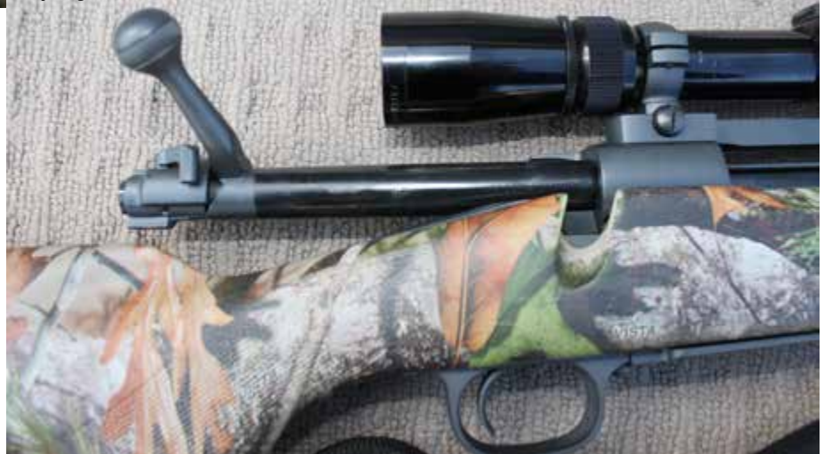
Micro Slick coating on the bolt is black and helped with noticeable improvement in cycling.
