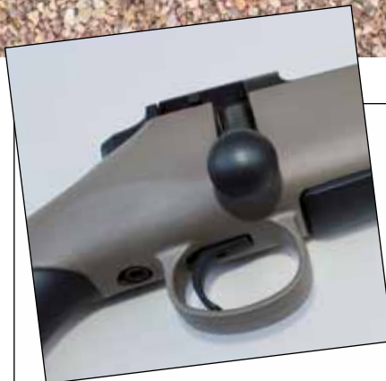
The triggerguard is integral to the stock design but allows ample access to the trigger blade.
