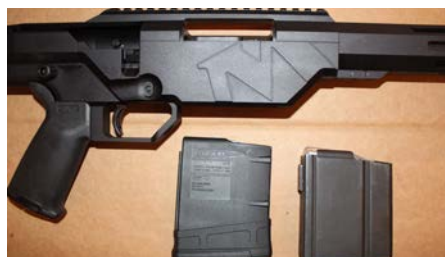
Like other MVP .308 case length variants, the Precision can use both AR10 and M14-style 10-round magazines.
