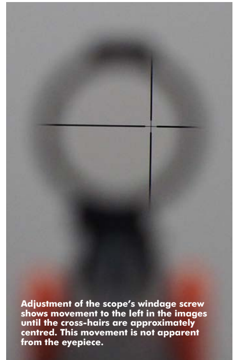
Camera view looking back through the objective lens from the muzzle showing marked displacement of cross-hairs to the right - but the view from the eyepiece would show them to be centred.
