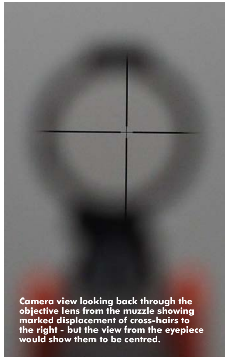
Adjustment of the scope's windage screw shows movement to the left in the images until the cross-hairs are approximately centred. This movement is not apparent from the eyepiece.
