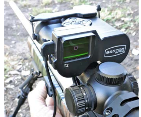
A rangefinding remote cable can be attached to the fore-end for ease of activation.
