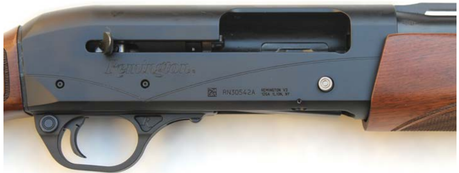
Right of the receiver shows ejection-loading port, substantial cocking handle and scalloped opening forward of the loading port so the cocking handle can be removed for cleaning.
