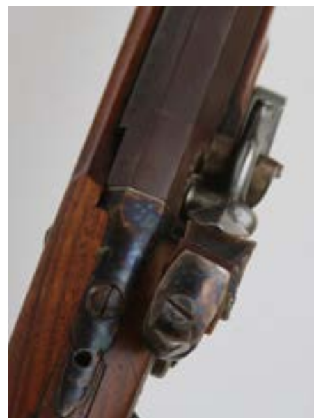
When clamped in, the cock the inside edge of the flint must clear the barrel otherwise it'll be deflected or broken as the cock moves forward under spring pressure.
