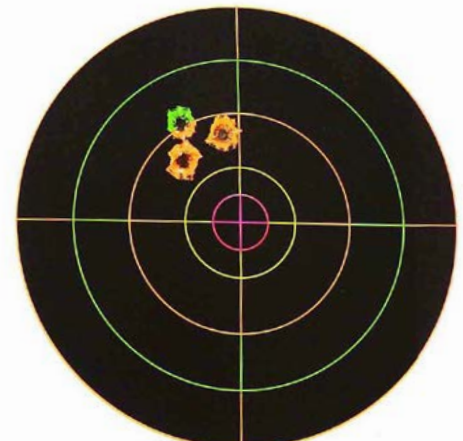
Bullet impact points were almost identical with muzzle brake fitted or replaced by the counterweight.
