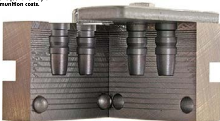
A bullet mould is just one way of saving on ammunition costs.
