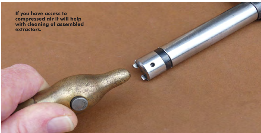
Cleaning tools help when removing compacted grease and powder residue from the extractor slots.
