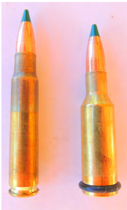
The long, slim cartridge gave better velocity for the amount of powder burned.
