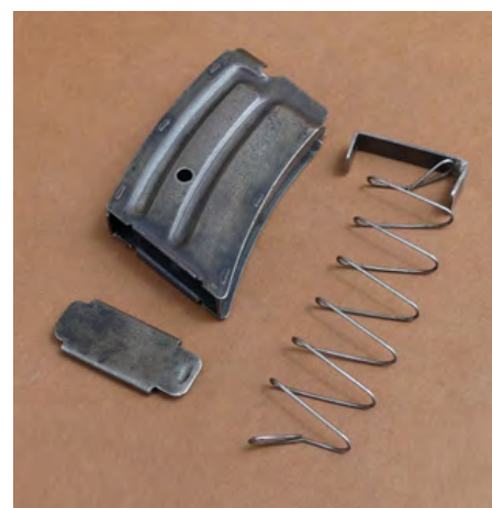
Cleaning dust and grease from inside magazines is best done when they're dismantled though some magazines may not be easily taken apart.
