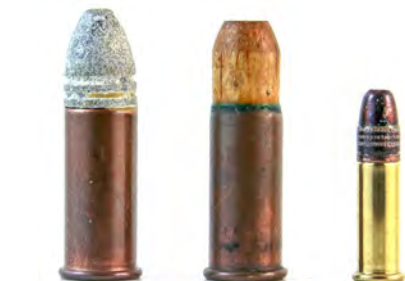
A standard .38 rimfire cartridge and wooden sabot shot load with a modern .22LR for comparison, both rounds having a 'U' headstamp from Remington.
