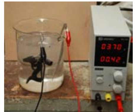
The electrolytic de-rusting process.
