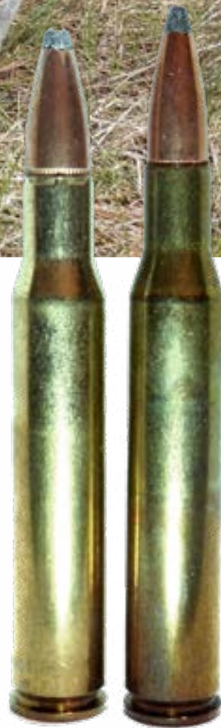
The .270 case (right) is the same length as its parent case, the .30-03, and as can be seen is slightly longer than the .30-06.
