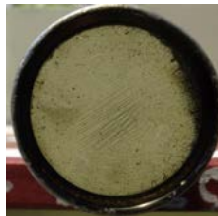
The ocular of an old Unertl Hawk, acquired for research, that's led a hard life. Not only has it a hairy fungus at the right but it seems the owner handled it with a rough glove.
