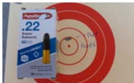
The twist-rate of the Weihrauch HW66 barrel couldn't sufficiently stabilise the heavier and longer 60-grain projectiles on the Sniper Subsonic loads.
