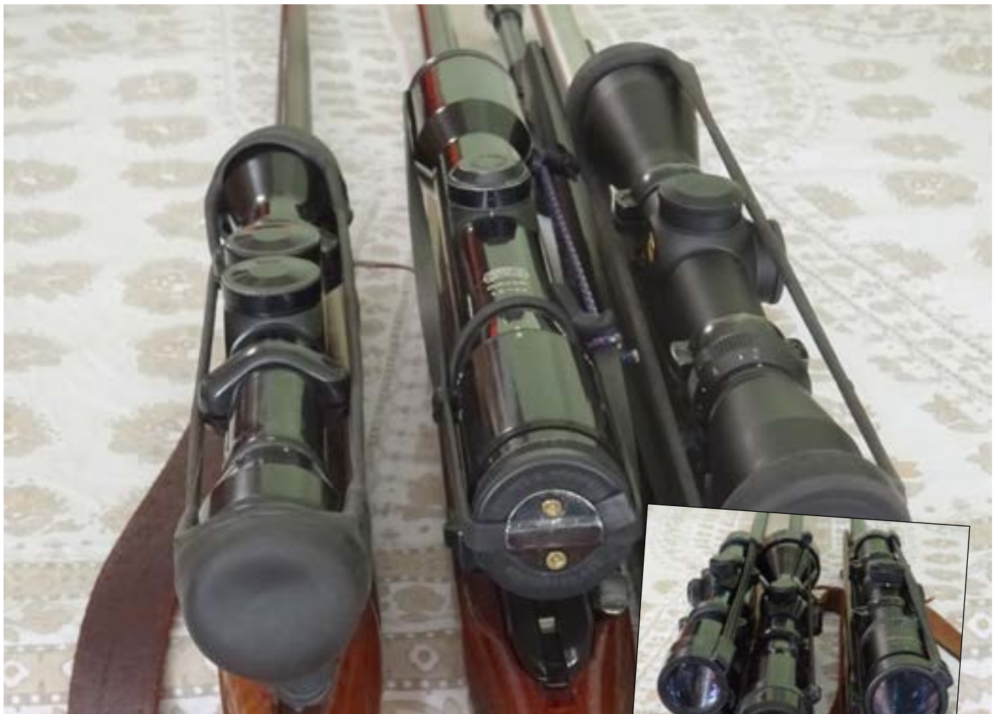
Two bikini covers with a much-repaired Uncle Mike's flip-off pair. The latter is quick to release but still not fast enough.
