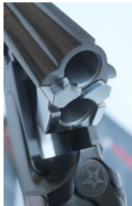
Super-strong ejectors and sturdy Boss locking system are great features.
