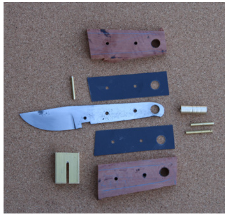
Component parts for a full-tang bunny knife. The slotted brass plate (bottom left) will become the finger guard, the squared notch behind the ricasso locates the guard where it will be secured with a brass pin and epoxy glue.
