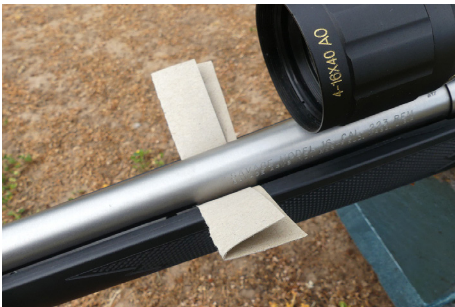
Floating barrels need sufficient clearance. The Savage is shown with a double layer of thin cardboard under its barrel.
