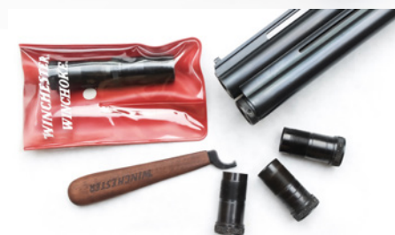
The Diamond Grade Trap gun had a fixed choke in the top barrel and interchangeable Winchokes below. Note collar on the end, berated at first but still very practical.
