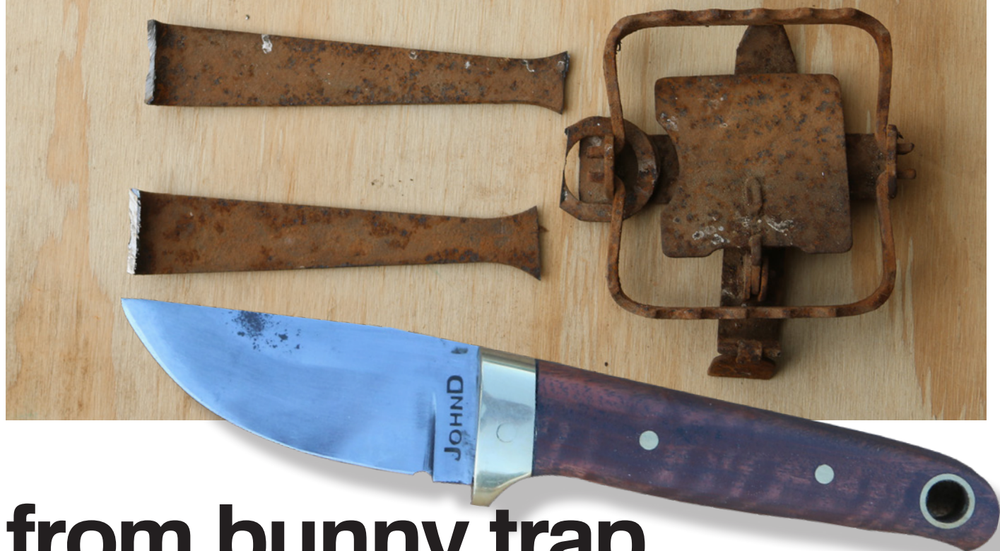
The spring from a trap like this has enough material for two small bunny knives.
