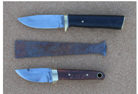
A half-tang design (top) allows a longer working blade.
