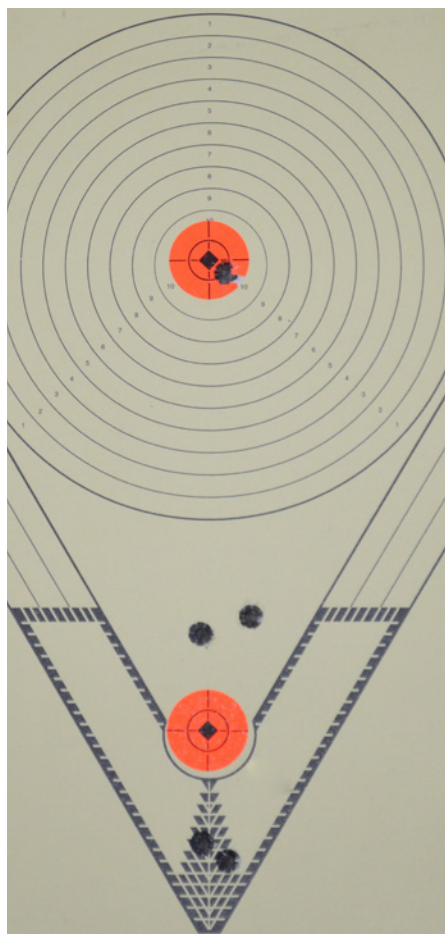
200m accuracy and turret precision/consistency test, executed after an hour of manual turret cycling from full-up/full-down and full-left/full right rotation.
