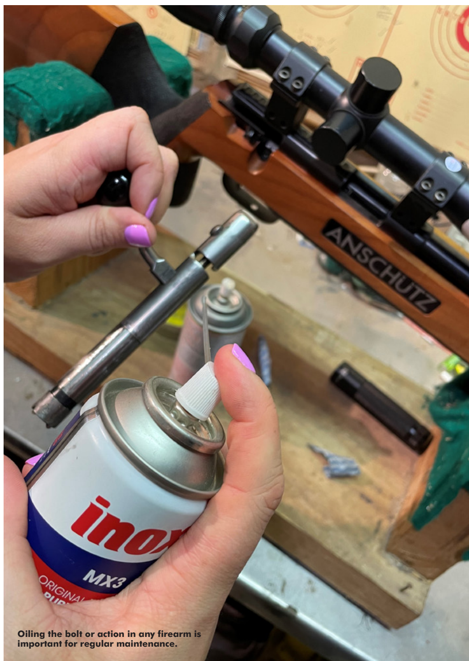
The bolt face on a bolt-action rifle often has wax build-up from ammunition and it's important to clean this and where the bolt face sits in the action.
