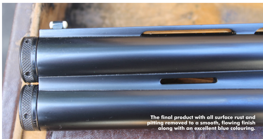
All rust and pitting have been removed.
