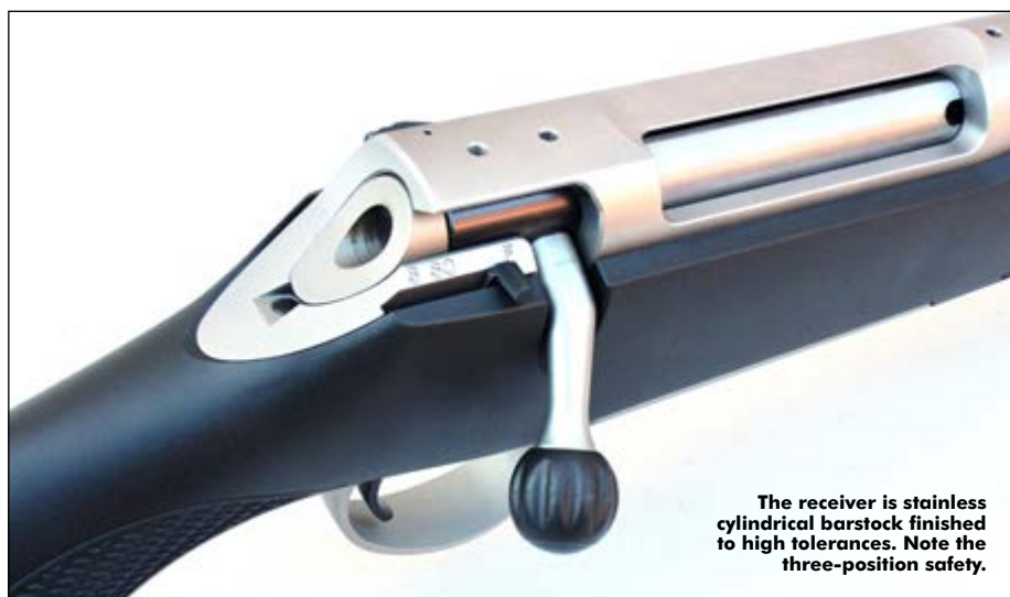
Well-profiled bolt release on the left of the rear receiver ring also acts as a guide for the bolt to travel on.
