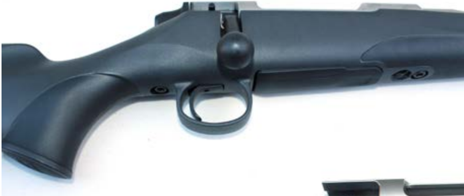
Action with straight bolt-handle and safety lever.
