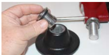
The Quick Trickle base plate is integrated for the bushing system.
