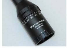
The ocular with adjustable eyepiece focus and power magnification ring.
