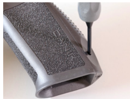
The Canik punch is used for changing backstraps.
