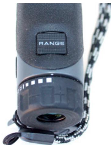
The 'power/range' button is easy to reach with the index finger, the eyecup with adjustable dioptre ring also evident.
