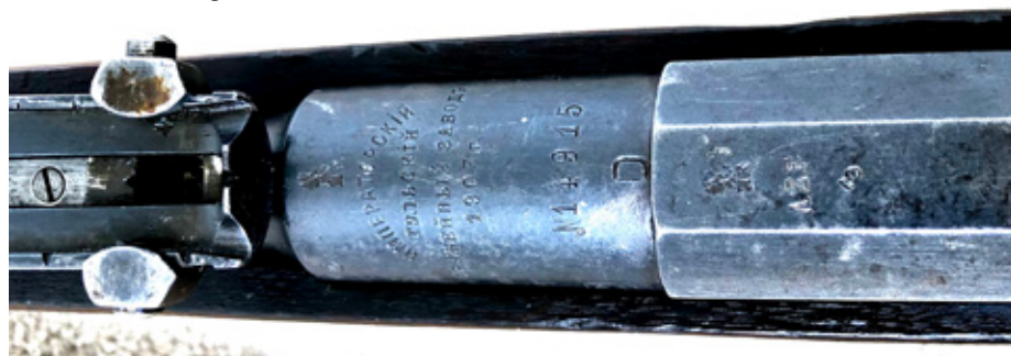
New Finnish markings (which correspond to old Arshin graduations).
