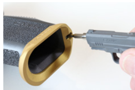
Mag-well removal using miniature Canik tool.
