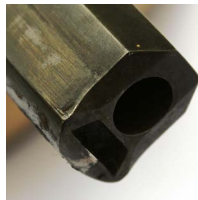
The breech end of the barrel showing a recess for the breech-locking bolt below the chamber, bevels on either side of the chamber allow the fingers access to the rim of a spent cartridge.
