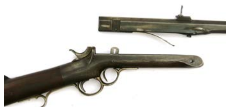
Rifle taken down to show the relationship between barrel and fore-end. The flat spring under the barrel tips the breech up when the action is opened.
