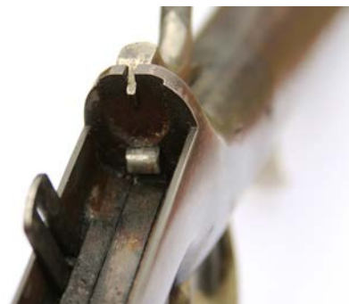
Wesson patented parts including wedge-shaped recess on the face of the standing breech, retractable locking bolt at the bottom and slotted link to the left of the receiver.
