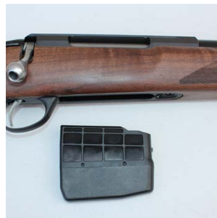
The 10-shot magazine (in .223 Rem) fits neatly in the well and clips into place securely.
