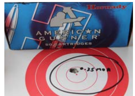
Outstanding accuracy with .308 Winchester Hornady ‘American Gunner’ 155gr ammo producing this ¼ MOA group.
