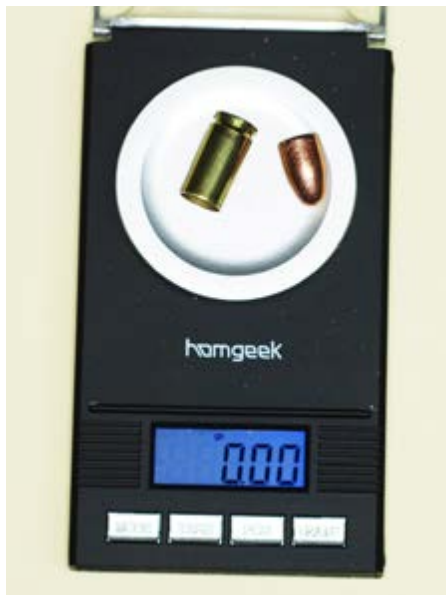
Primed case and projectile on the scale, zeroed so the display reads 0.00.
