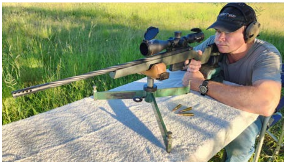
Spiral fluting matches nicely to spiralled holes of the muzzle-brake while the bold chin (fore-end) of the Range XP says it's part of the Weatherby family.
