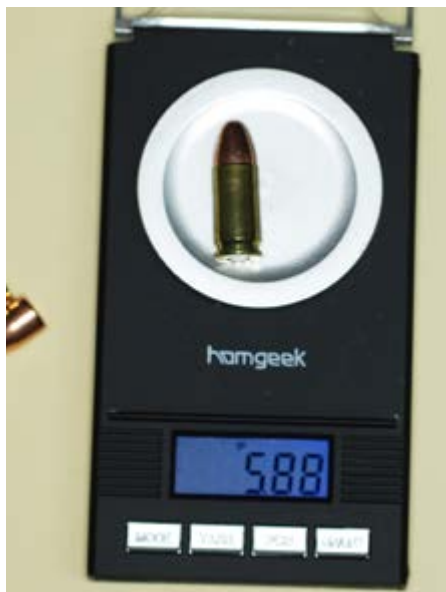
Loaded round placed on the scale shows only the difference, namely the powder charge, which in this round should be 5.8 grains.
