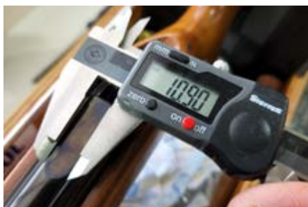
The receiver dovetail must be measured before choosing the rings.
