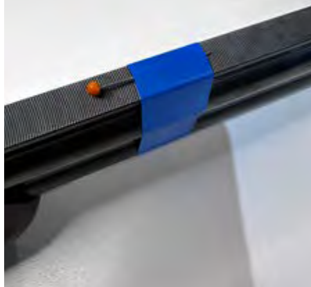
To create a temporary centre bead, insulation tape and a sewing pin can be used.
