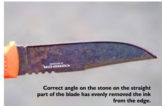
Use a dark marker so you can easily distinguish between parts of the blade that do and do not have ink on them.
