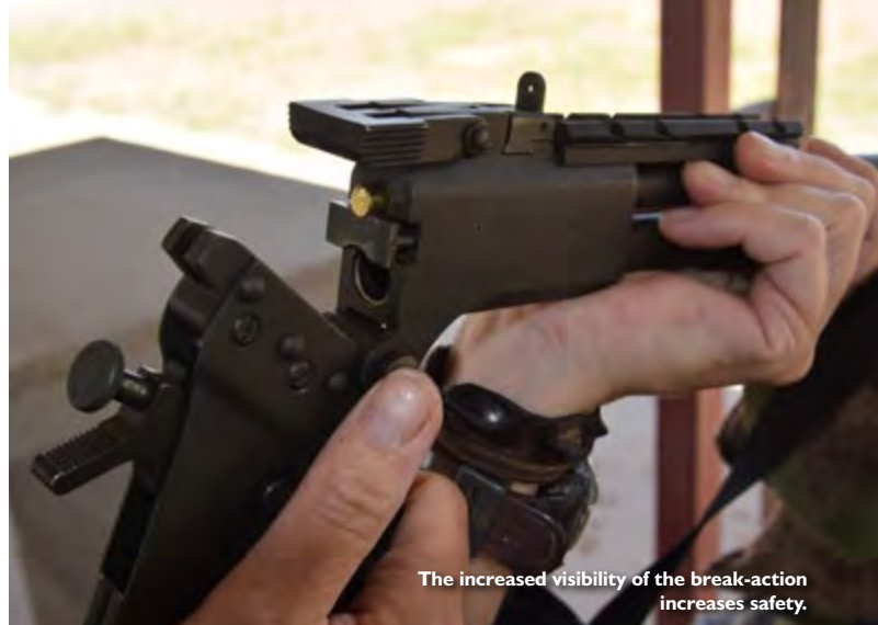
Note the hammer and the knob which is used to select the barrel.
