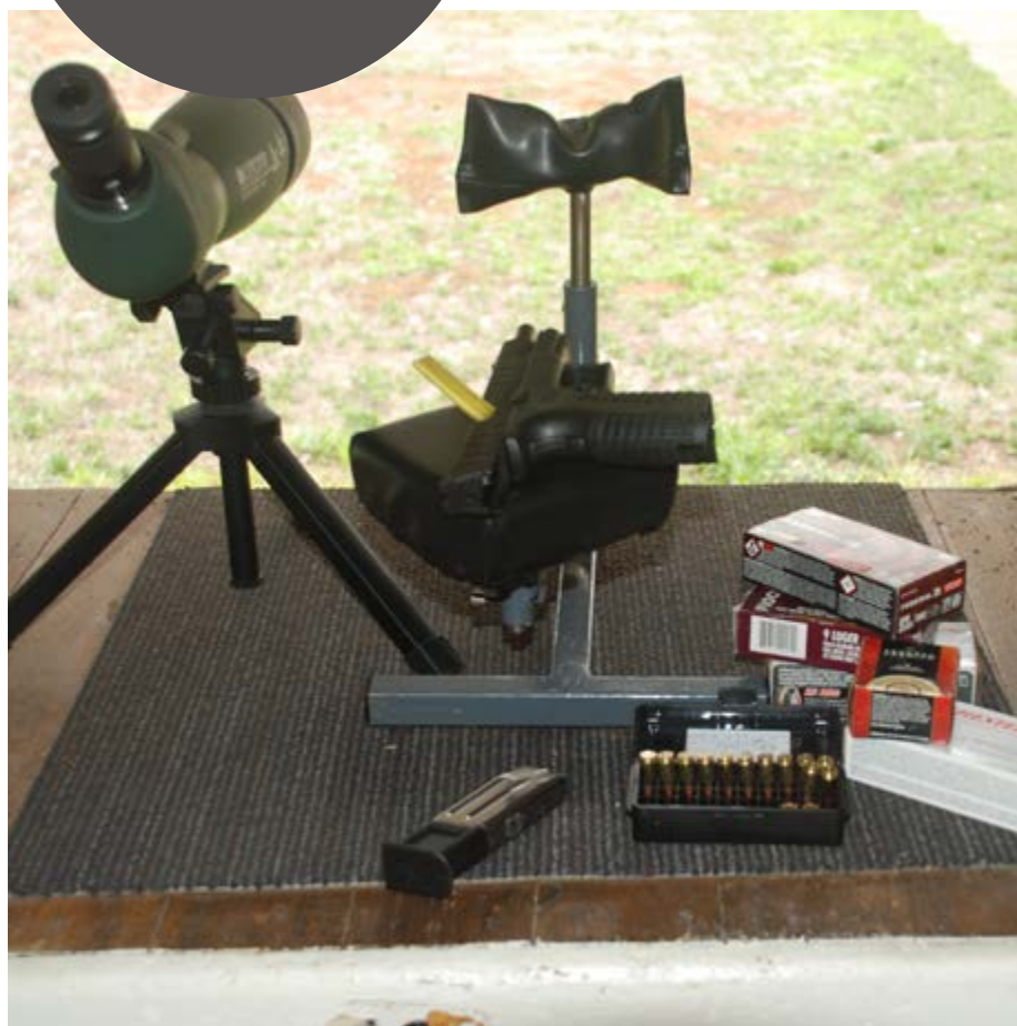
Bench tests used six different loads, all of which cycled well and performed flawlessly.
