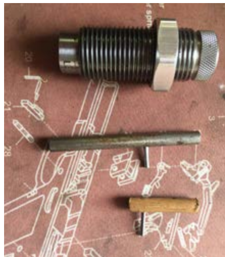
John uses a .308 Winchester Lee factory crimp die for his loads, using a length of quarter-inch steel rod. Proper length was determined by trial and error using quarter-inch dowel.
