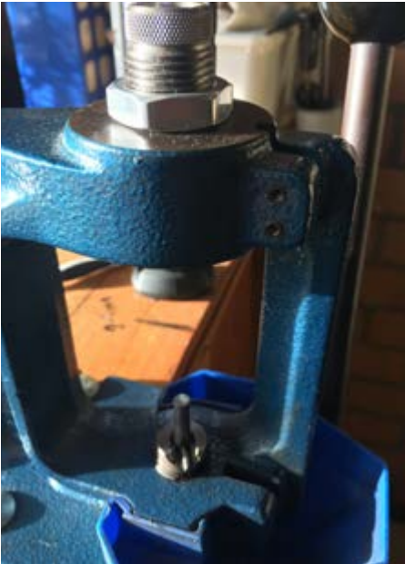
The Lee factory crimp die in use with cartridge support in the author's old Simplex press.
