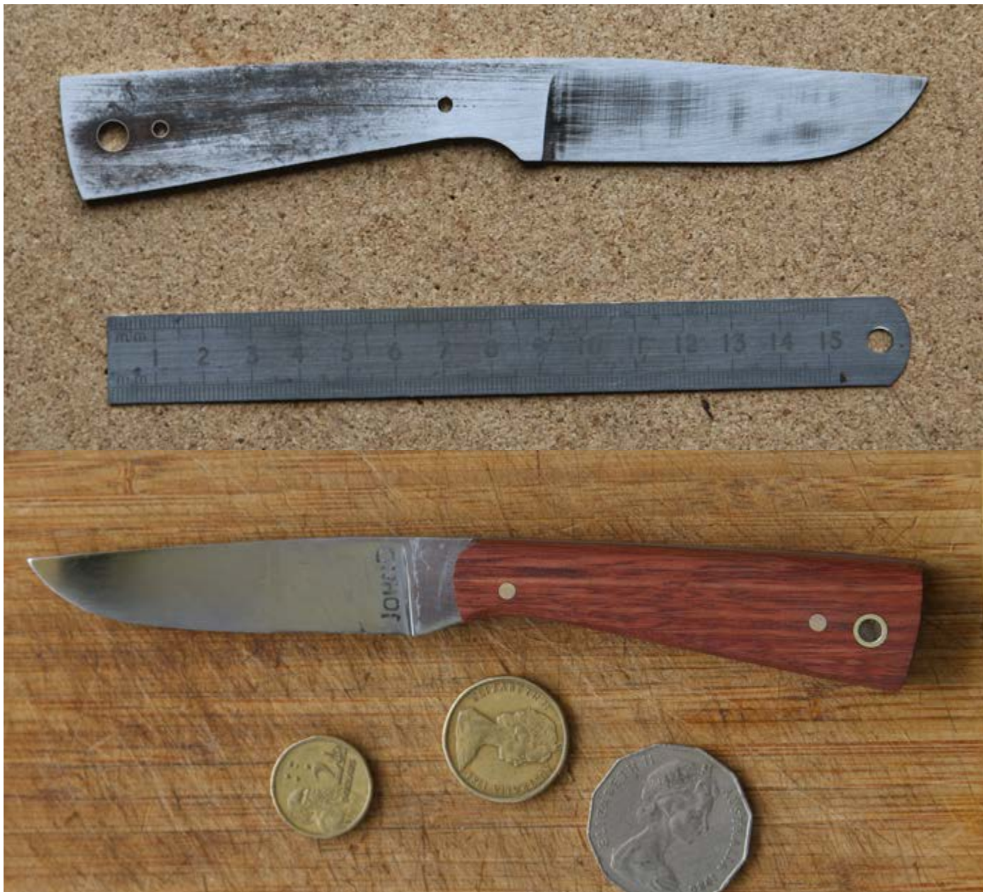
Top; The blank almost ready for heat-treating with holes drilled in the tang and bevels ground. The blade should be polished before heat-treating. Bottom; The finished article - a simple little knife.
