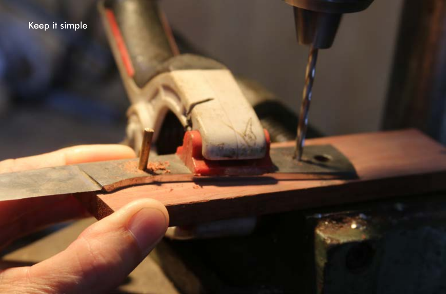
Drilling the holes in the handle scales. Note pin inserted in hole on the left to ensure the second pin hole and lanyard tube hole line up.
