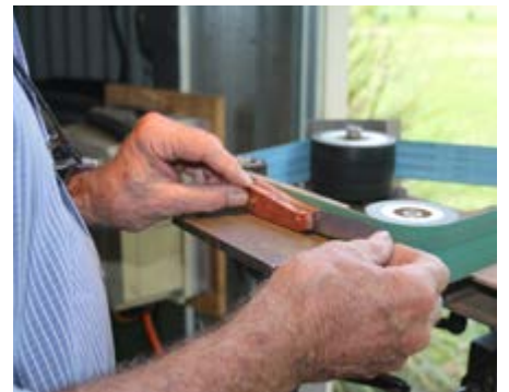
Shaping the handle on the grinder.
