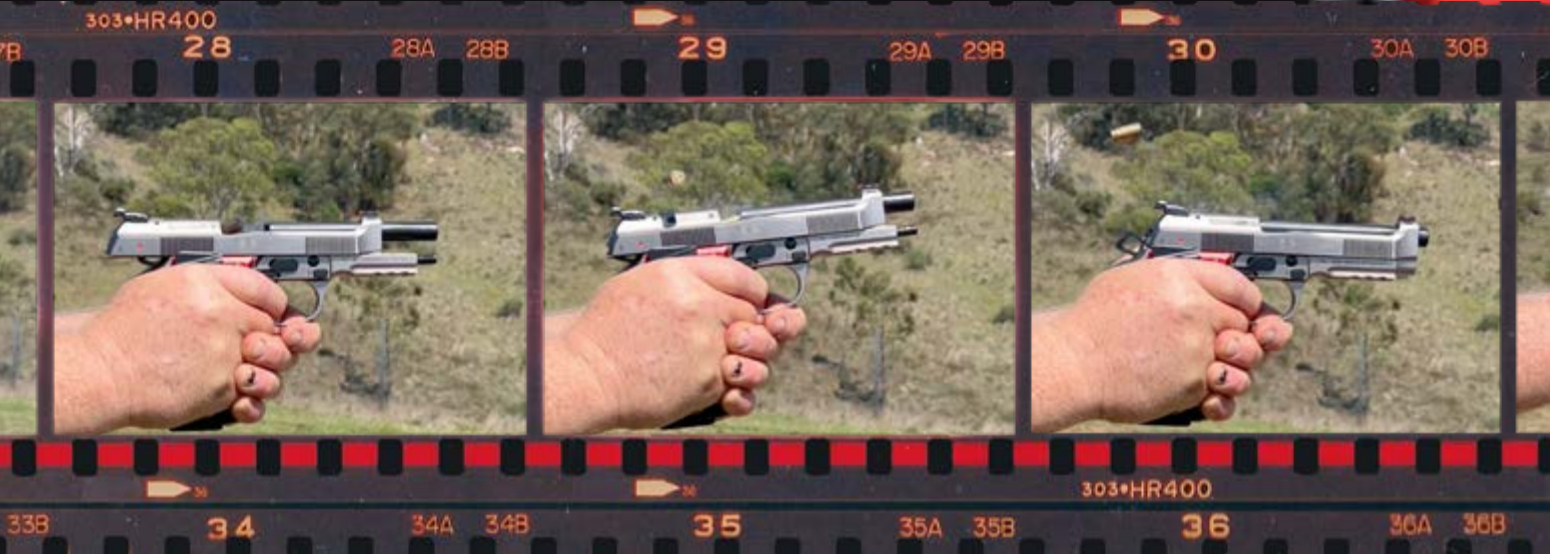
The 92X milliseconds after firing the cartridge extracts. Under recoil the case ejects and a new round is chambered. As the spent case flies the 92X is already back on target.
