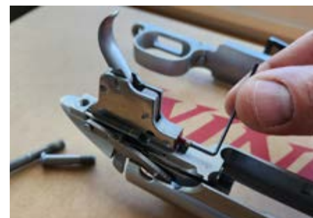
Trigger adjustment made easy with the turn of an Allen key.
