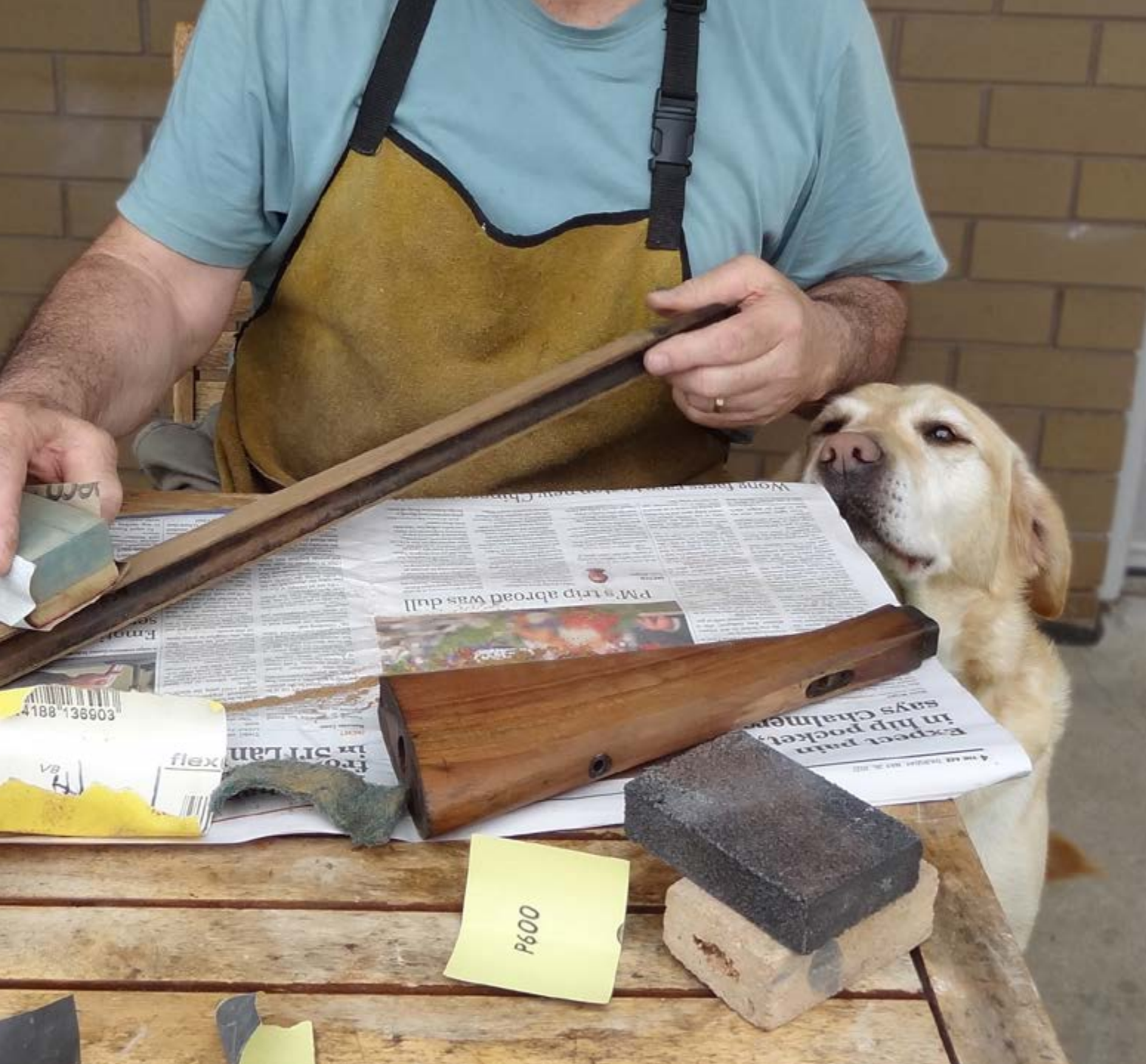
Removing surface rust using wet and dry sandpaper.
