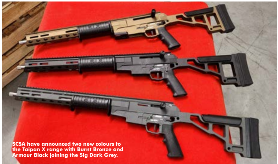
The new Taipan incorporates a left-side receiver slot and charging handle.
