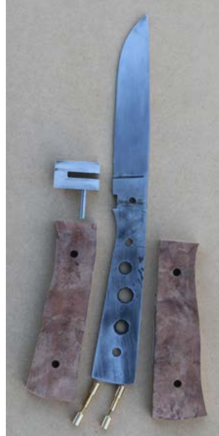
Though they vary in size, component parts of the Millthorpe Hunters are the same. This is a small Hunter with 10cm blade. Handle material is NT ghost gum, brass Corby bolts to attach the scales and a 416 stainless steel finger guard and pin.
