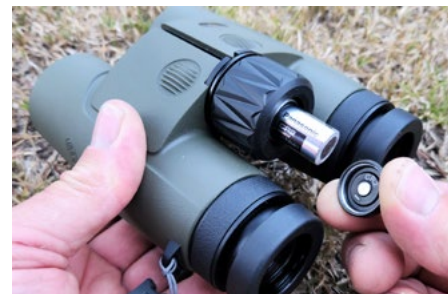
The battery compartment on the 10x42LR is neatly housed within the focus wheel and O-ring sealed to be waterproof.
