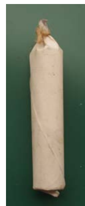
Completed Pritchett cartridge containing a .55" projectile.
