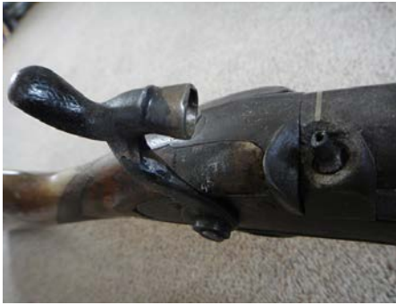
Shrouded hammer (replaced), 'fence', nipple and silver washer between barrel and breech plug.
