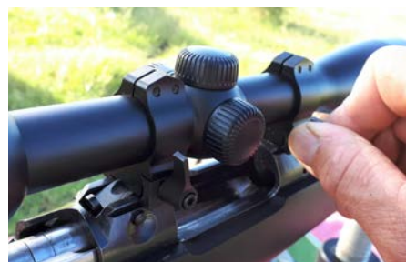
Tighten all screws after adjusting the cant alignment and thumb-tighten QD levers securely to the receiver.
