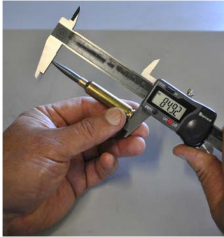
Vernier calipers (digital) are commonly used by shooters for basic measurements. In this case it's cartridge overall length and assessing 'jump to the lands.'
