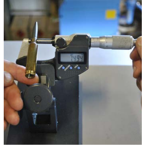
A digital micrometer used to measure case neck dimensions to assess consistency and chamber clearance.
