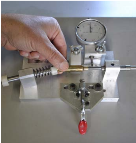
A runout gauge used on a dummy cartridge after chambering can tell a shooter how the cartridge is being presented to the bore.
