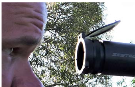
Ensure correct eye relief prior to tightening of all ring screws.
