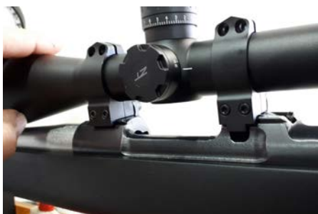
Place the scope in the rings and locate to the receiver dovetail.
