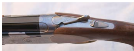
The top lever and tang demonstrates the wood-to-metal fit along with red dot in the barrel selector-cum-safety catch for easy identification of which barrel is firing first.
