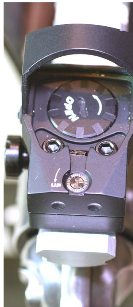
Top of the unit houses the elevation adjustment screw and battery cap.
