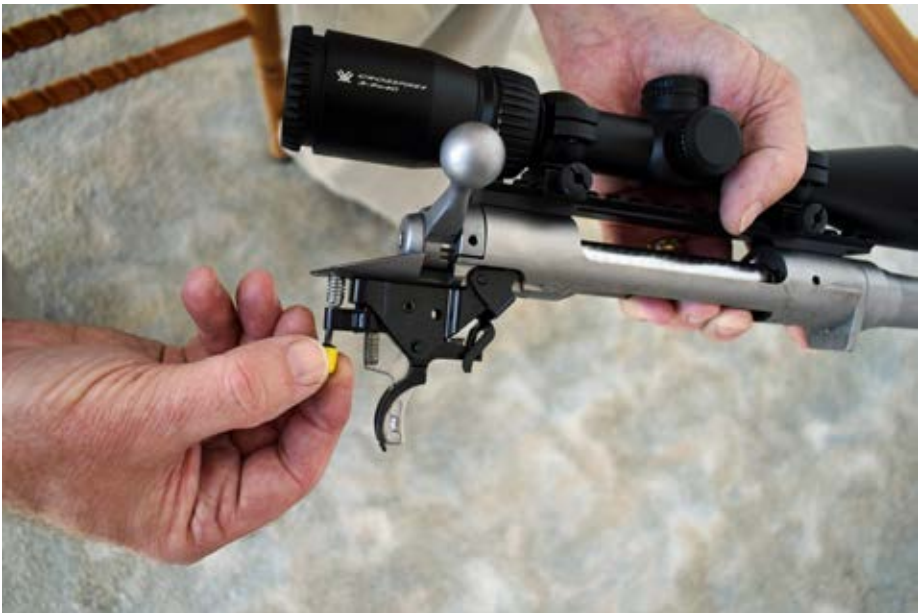
The AccuTrigger is adjustable for weight-of-pull.
