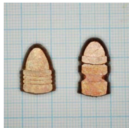
The 'smash' test shows whether the coating has properly bonded to the lead.
