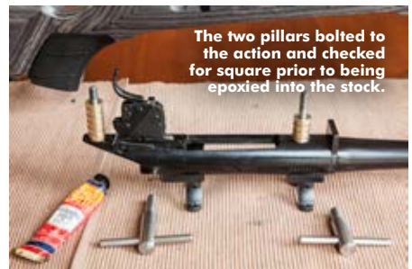
The slow-curing J-B Weld, along with the other consumables, produced an effective result.
