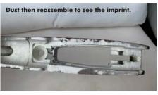
masking tape between the fore-end and top wood on the flats where the two timbers meet. The idea is that once dried and tape removed, upon reassembly the RTV should clamp down tightly around the barrel, providing support and rigidity.
