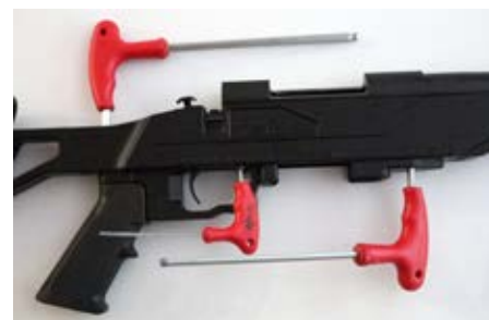
The final step is fitting up the magazine and grip adapters (hex keys show bolt locations).
