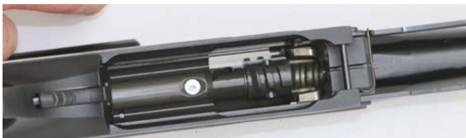
View through the magazine well. Bolt body on left, pinned to rotating bolt head ready to turn into the breech shroud via an interrupted thread.
