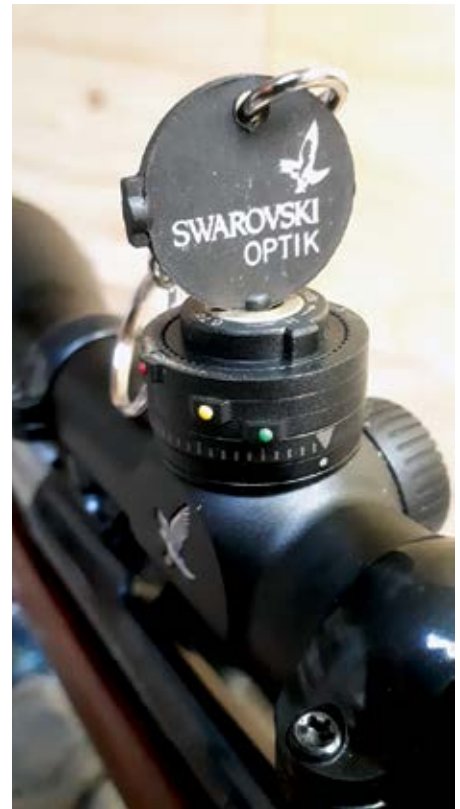
Adjusting the BT and removing adjustment cap with the supplied tool.
