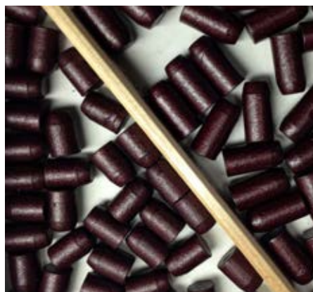
Bullets with final coat baked on.
