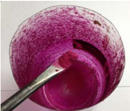
Adding powder to the cut-off HDPE bottle.
