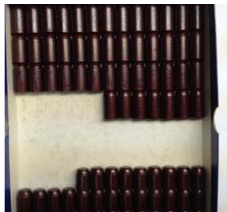
Completed bullets after swaging.
