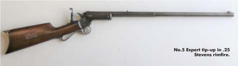
The steel No.5 action was originally nickel-plated as the remnants show. The small rectangle near the top rear of the receiver is the locking lug, activated by the locking button on the left. The tang sight is a No.1 Lyman Combination, not original to the rifle but contemporaneous.
