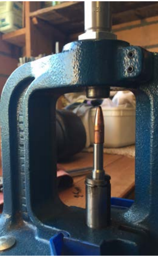
A .338 projectile goes into the Lee resizing die.
