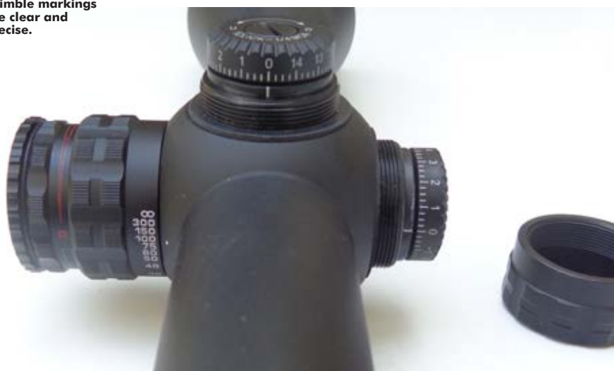
Remove the centre screw and slide off the thimble to set new zero.
