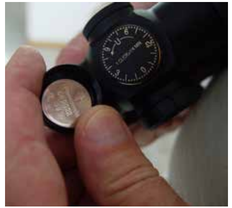
Illuminated reticles use batteries that can go dead in the field.
