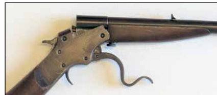
Marksman No.12 action open showing similarities to the Maynard patent rifle it was based on.
