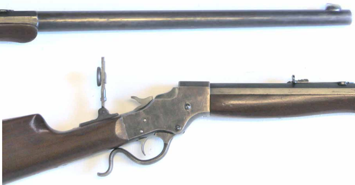
Stevens Ideal No.44 rifle in standard centrefire configuration had a barrel 51mm longer than the rimfire version.
