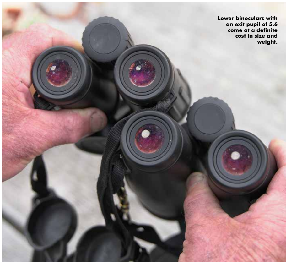
10x42 compared with 8x32, considerable size difference but both with exit pupil of around 4.
