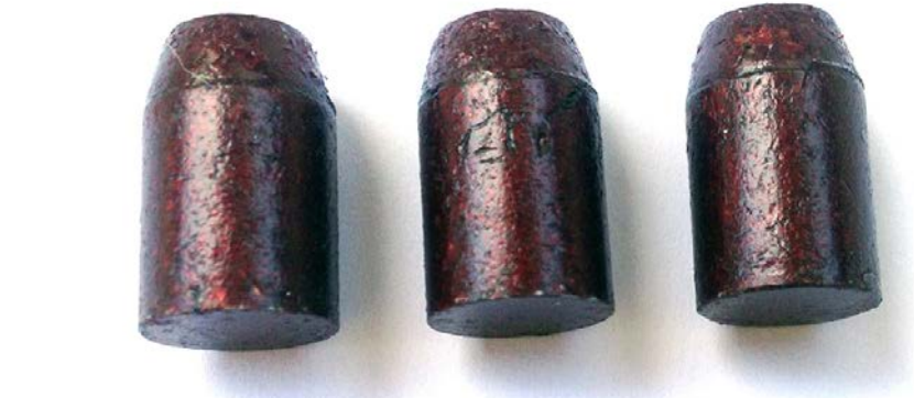
Plain base 154-grain coated bullet that shot well at 25yds.
