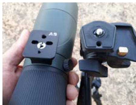
The \frac{1}{4} " UNC female thread on the spotting scope (left), plus tripod mount attachment with male thread.
