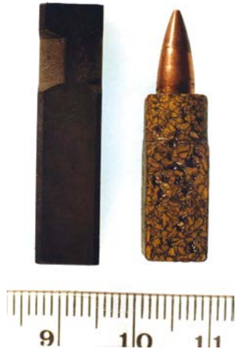
Fig 1: Two combustible cartridges at different stages of development. Left: an early, partly successful pattern. Right: the final H&K 4.75x23.
