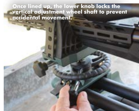
On the DFT 2 the rear foot is adjustable via a large easy-to-use turn knob for vertical adjustment.
