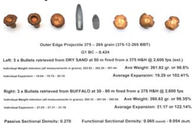
Photo 2: The 375 265-grain OEP recovered from sand and a buffalo.
