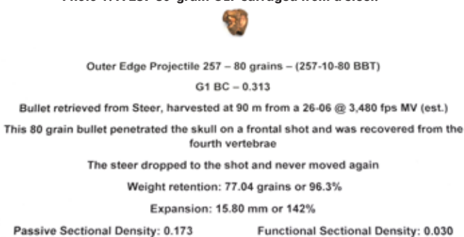
Photo 1: A 257 80-grain OEP salvaged from a steer.
