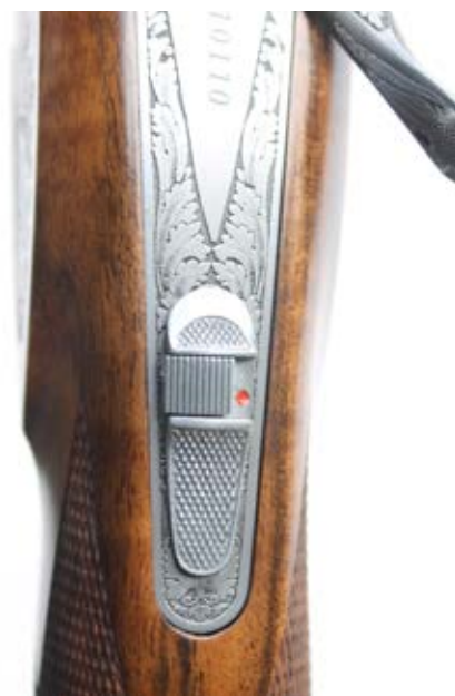
Design of the barrel selector-cum-safety catch allows the top lever to be operated without interference from the catch.
