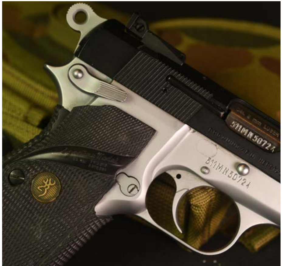
The safety lever is on both sides of the slide and can be operated with either hand, though the magazine release button is on the right.
