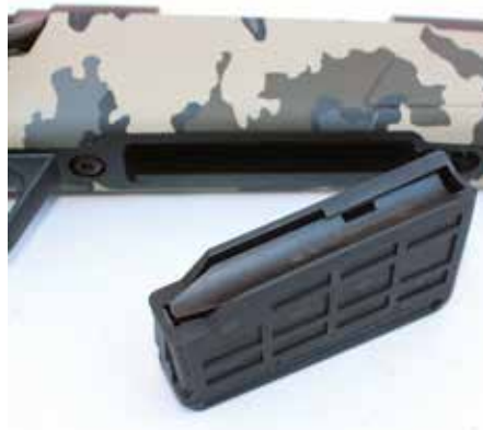
Detachable polymer magazine with single-stack configuration held three rounds in .270 Winchester.
