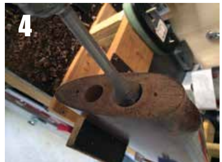
Don't apply too much pressure when boring the hole.
