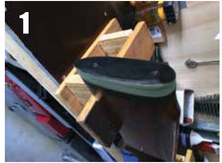
Secure the action in a vice. Don't overtighten and use soft guards on the jaws to avoid marking.
