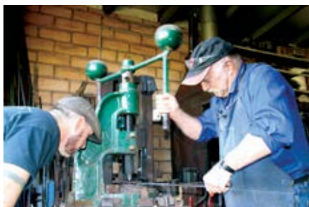
Putting the hammer finish on the blade with the fly press.
