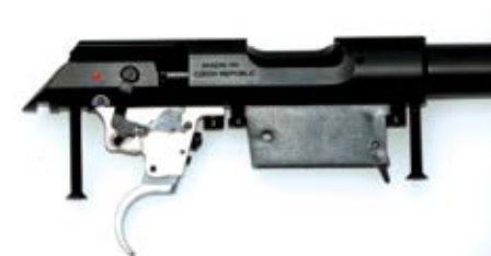
Right side of receiver showing location of the safety lever.
