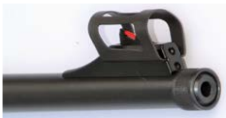
Front of the barrel showing adjustable foresight and bevelled muzzle with threaded end.
