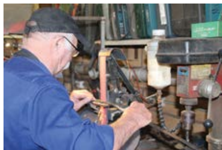
Finishing the blade shape on the belt grinder.
