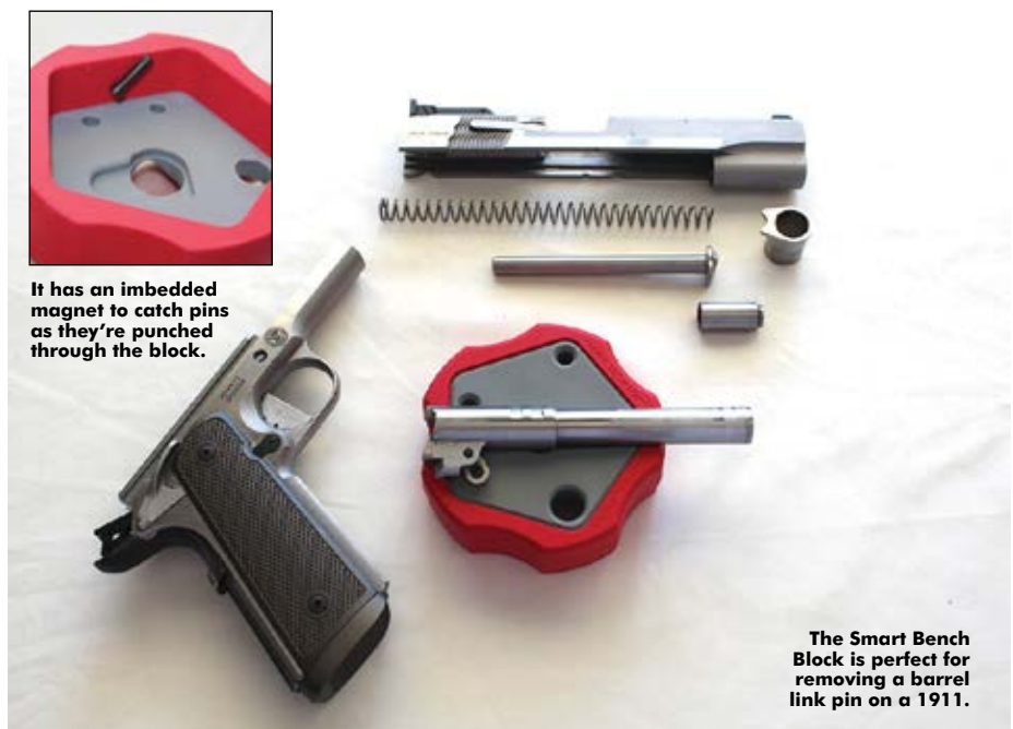
The Smart Bench Block has a 1911 Barrel Bush tool moulded into the base.
