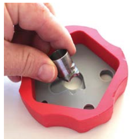
The Smart Bench Block has a 1911 Barrel Bush tool moulded into the base.
