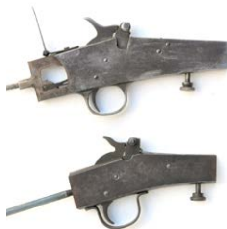
The No.6 (top) and No.6 Improved actions compared.
