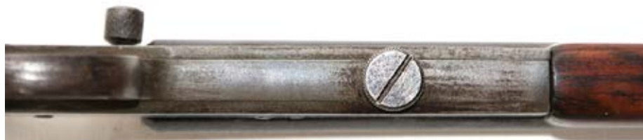
Bottom view of the receiver showing the laminated construction. The slotted screw head is the take-down screw.
