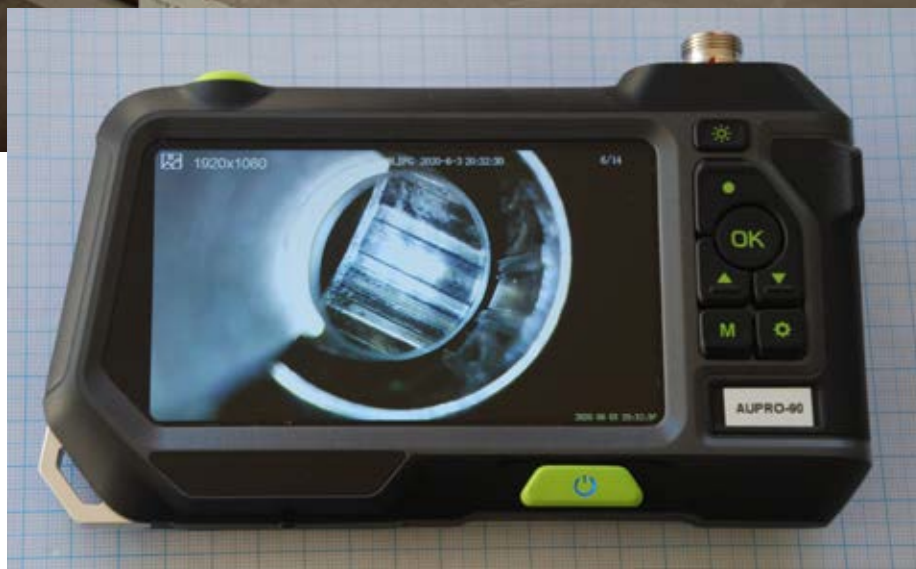
The display can call up images with probe disconnected, in this case showing the muzzle of an Enfield .380 revolver.
