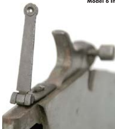
Pressed metal tang sight used on the No.6.
