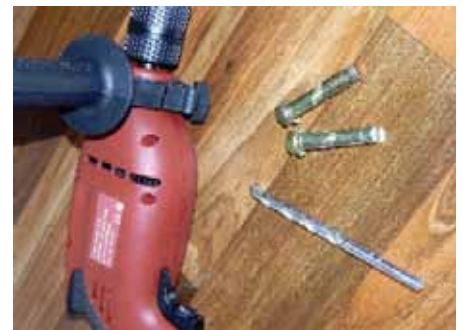
It is a simple procedure to bolt down a safe. All that is needed is an impact drill, some dynabolts and the correct size masonry bit. A piece of electrical tape wrapped around the bit at the correct depth will tell you how deep to drill.
