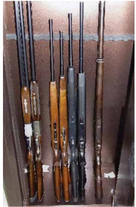
The finished item. Some form of gun-rack inside the safe is necessary to prevent guns from falling over. Since this photo was taken, Craig Richards has added a rubber floor mat for the same reason. The things in the bottom are sachets of silica gel to absorb moisture from the air within the safe to prevent rust.
