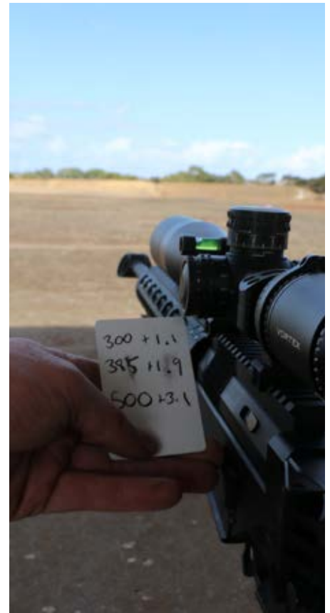
A dope card being stuck to the rifle, left column distance, right for clicks.
