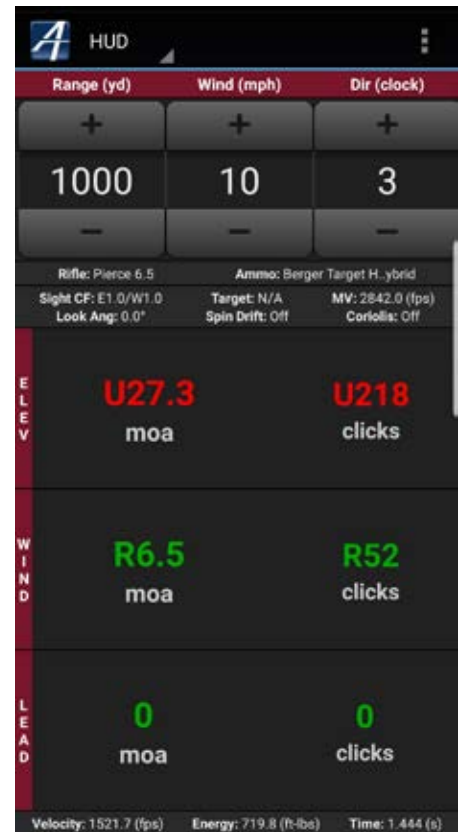
Steve used a phone app called Applied Ballistics to calculate exactly how many scope clicks were needed to hit the targets.
