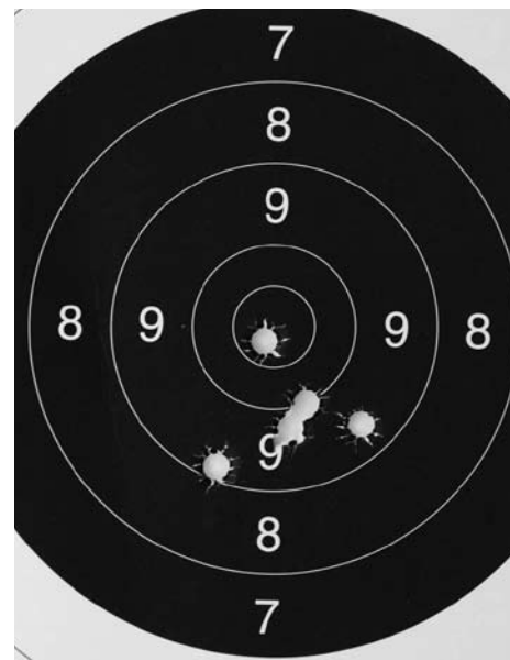
This is a target with five shots from a .44 Magnum at 25m. The shots are well within the 3" circle.
