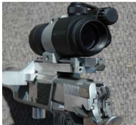
The direction lever (centre under the rear optical lens) is moved to compensate for the lead required on the moving target.
